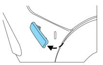
3. Remove the bulb socket from the lamp assembly by turning it counterclockwise.
